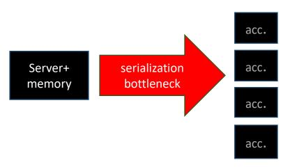
(a) Serializing data from main memory to accelerator memory, over e.g. PCI, may slow down the performance of multithreaded accelerators, such as GPUs with thousands of cores.
