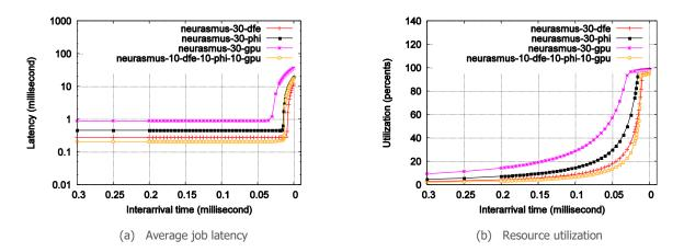
Figure 8: Performance of Neurasmus workload on deployments using only DFEs, Xeon PHI and GPUs, as well as on mixed deployments.
