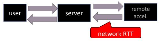
(b) Accessing a remote accelerator over an uncongested network may not necessarily increase the transfer time, as compared to accessing the accelerator locally through PCI, but introduces an latency round-trip time overhead, which is independent of the task data size.
