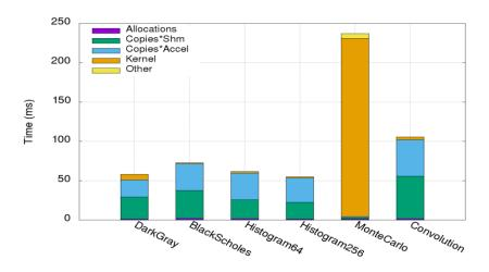
Figure 9: Latency breakdown when executing various computation kernels in GPUs.
