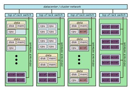
(b) accelerators as independent, shared resources in a disaggregated rack
