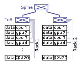
Figure 15: A uniform deployment of accelerators inside two racks.
