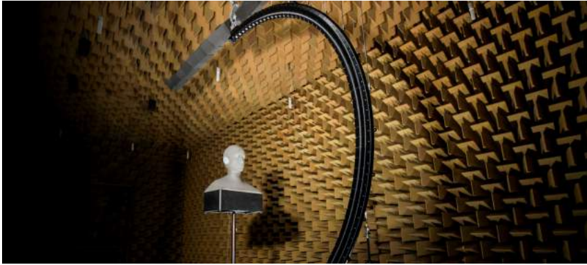
Figure 4.1.: Measurement setup of the arc and an artificial head on a rotating turn table at ITA, RWTH Aachen University.
