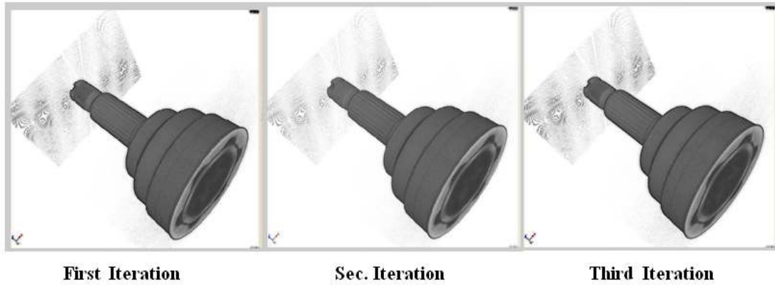
Fig. 13. Noise suppression by the iteration technique
