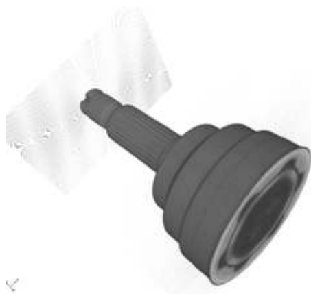
Fig. 4. NT of a CV car joint. The noise is clear at the top part of the image. The noise was arising from the reconstruction technique
