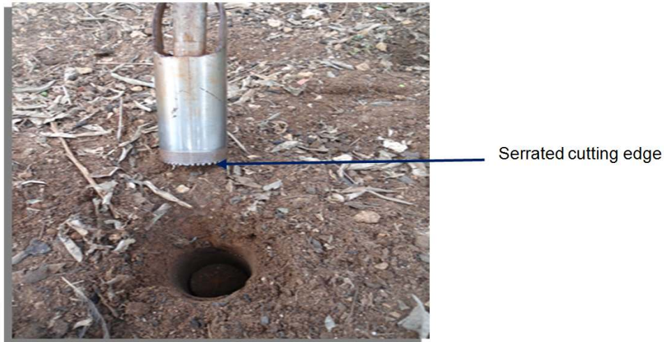
Fig. 2. Part of root sampling soil auger with serrated cutting edge
