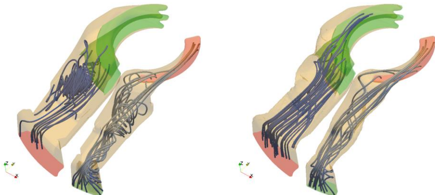
Figure 8. The left and right figure represents the streamlines for the baseline and optimized ducts. The optimization was clearly successful as the recirculation zones have all but disappeared.
