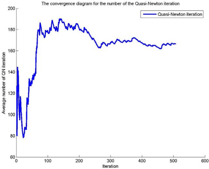
Fig. 4. Monte Carlo simulation of the number of quasi-Newton iteration for curve fitting of Price_1k_v2
