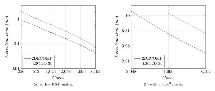
Figure 15: Execution time of complex to complex homogeneous FFT on Curie using 2D decomposition scheme and saving transpositions
