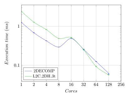
Figure 13: Execution time of  $256^3$  complex to complex heterogeneous FFT on Edel and Genepi using 2D decomposition scheme and saving one transposition
