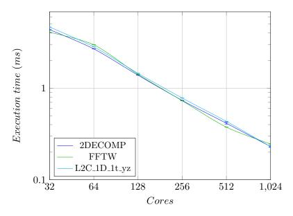
Figure 14: Execution time of 1024<sup>3</sup> complex to complex homogeneous FFT on Curie using 1D decomposition scheme and saving transpositions
