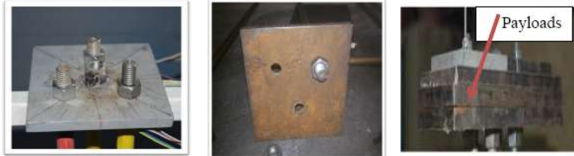
Plate 6: Steel plate used as pile cap and payloads.
