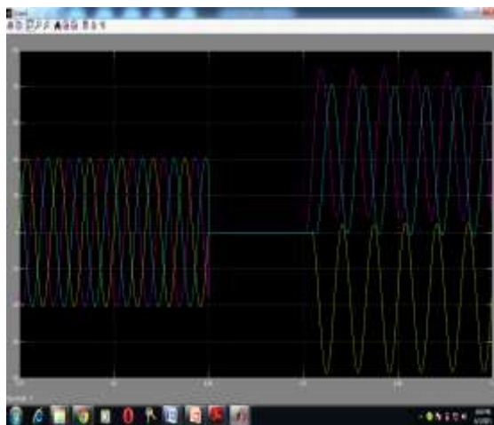
Fig 5. Output voltage with 3 phase fault
