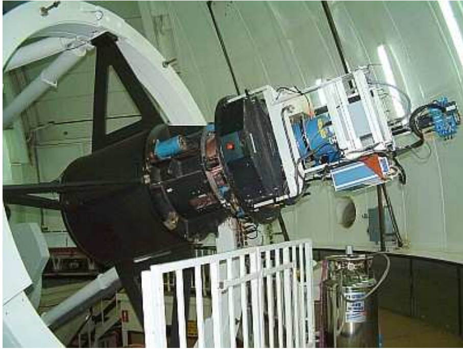
Figure 2.2: The WFC mounted at the prime focus of the INT. The telescope is in the park position where it may be filled with liquid nitrogen which is used to cool the instrument. The dewar for filling the camera with the coolant is below the instrument in this image. The image was taken from the website of the ING group of telescope a .
