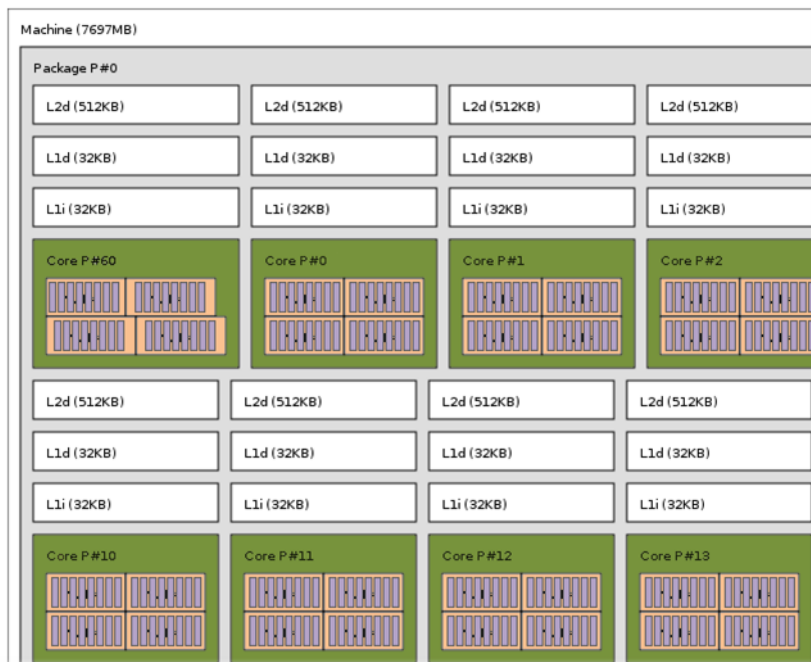
Figure 3.5: Possible mapping of blocks, threads and elements to the compute and memory hierarchy of a Intel Xeon Phi . Blocks are mapped to cores, threads to processing units and multiple elements are executed per thread.
