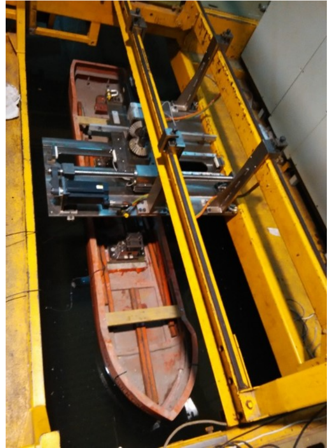
FIGURE 5. Ship model attached to PMM setup
