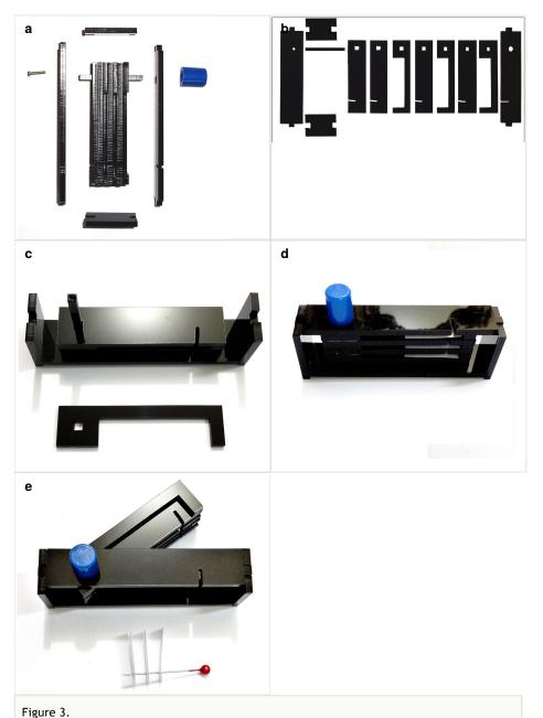
Step-by-step of construction of the pinning block mechanical.
