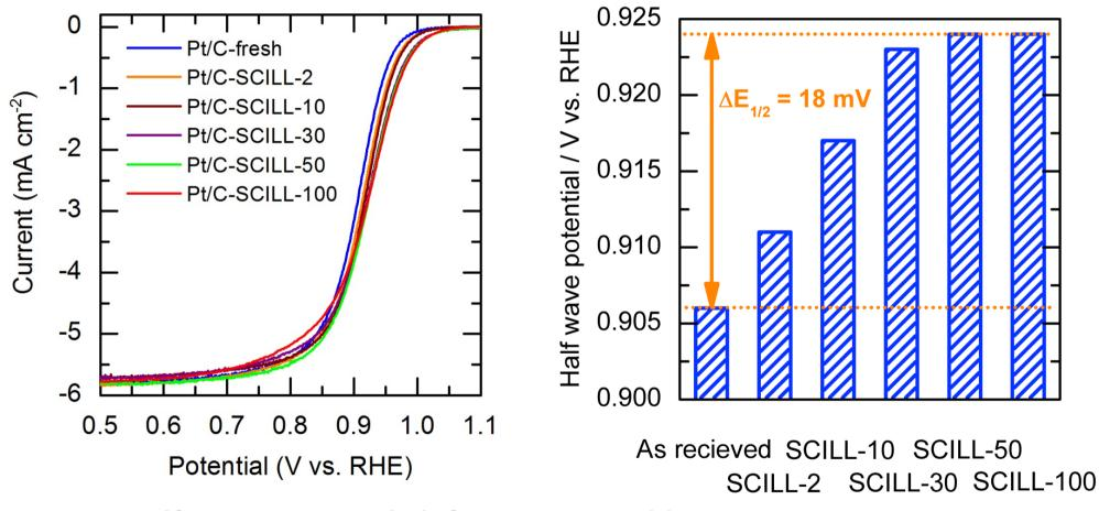
Half wave potential shifts pronounced by 18 mV
