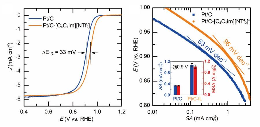
Pt/C-[C<sub>4</sub>C<sub>1</sub>im][NTf<sub>2</sub>] exhibited the highest activity towards ORR, which is three times more active than the pristine Pt/C
