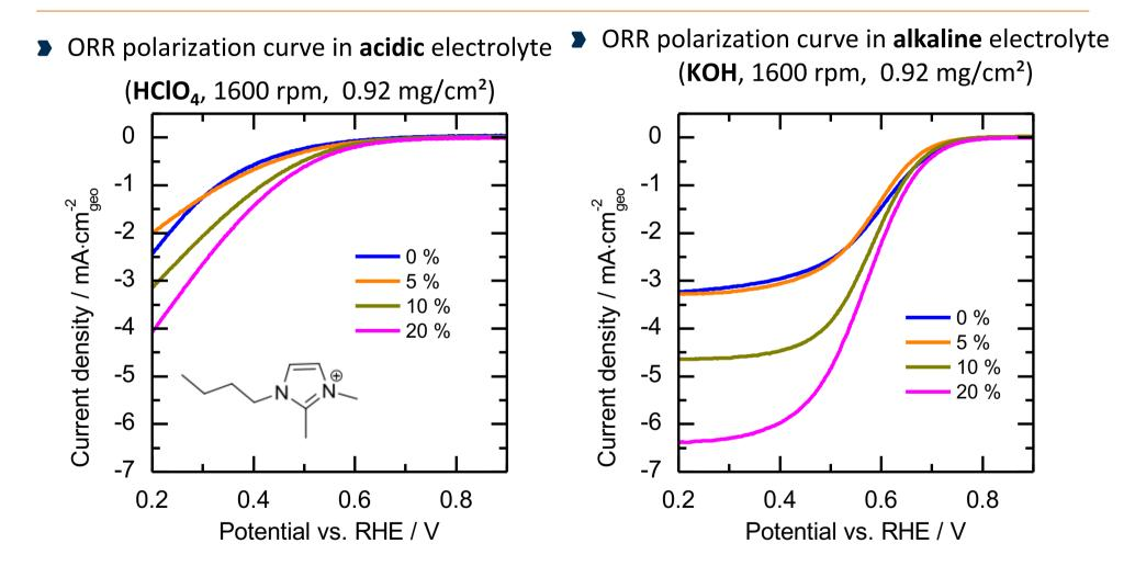
**[BMMIM]**[NTf<sub>2</sub>] can boost the activity of N-Doped carbon in acidic and alkaline media
