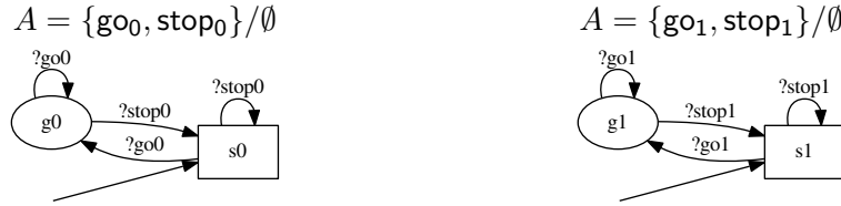
Figure 4.9.: Refinements S_0 and, respectively, S_1 of the signal design (A) up to renaming of actions.
