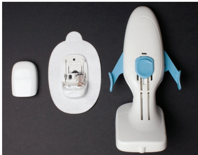
Figure 1: CGM system components: transmitter, sensor base, sensor inserter (from left to right).
