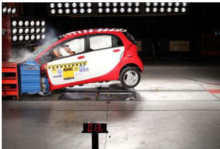
Figure 2: Mitsubishi i-MiEV – 64 kph frontal offset crash test
