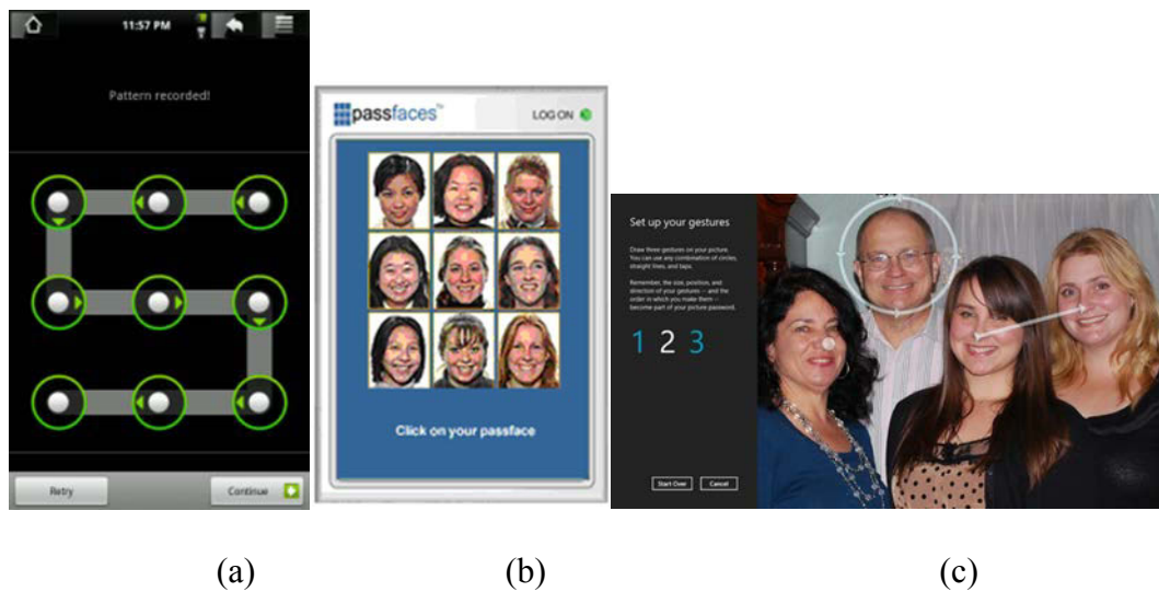
Fig. 1 – Examples of existing graphical password schemes (a) Android Unlock Pattern (b) PassFaces (c) Windows 8 Picture Password
