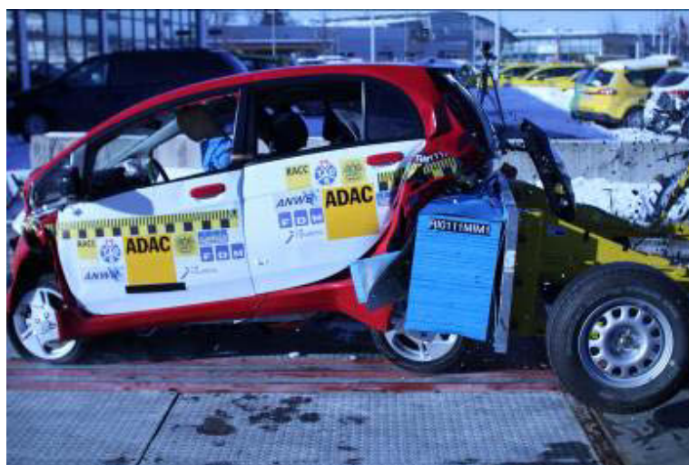
Figure 4: Mitsubishi i-MiEV – offset rear impact according to U.S. standard test procedure at 80 kph
