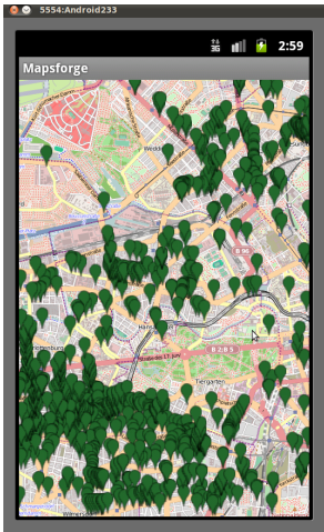
(a) Points of Interest: too many overlapping markers make the underlying structure of the region invisible
