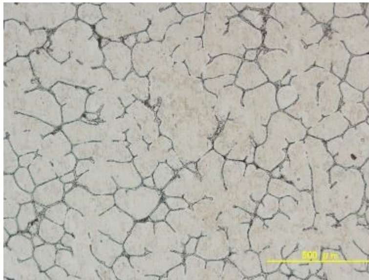
Fig. 5.17: Microstructure obtained by the quench test (quench temp.: 590 ^{\circ}\text{C} , cooling rate before quench: 0.24 K/s).
