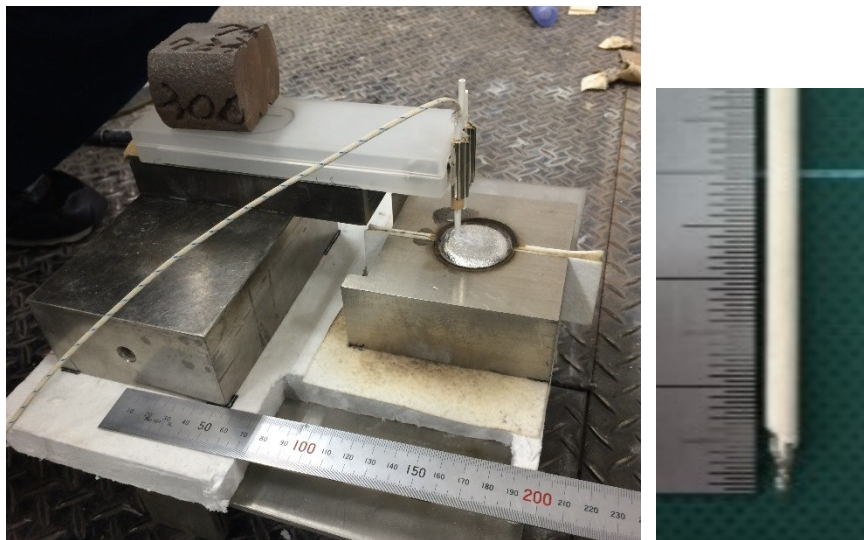
Fig. 5.16: Method of fixation of thermocouple: (left side) enlarged view of the thermocouple end.
