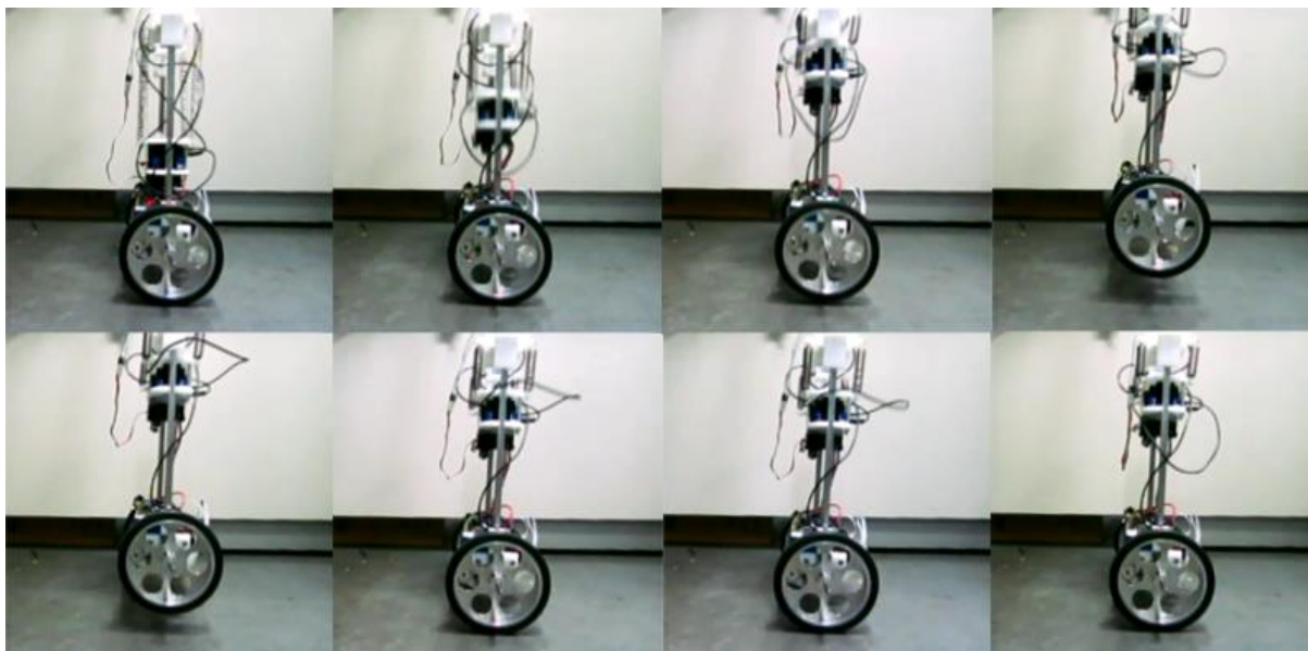
Figure 5-16: Hopping motion demonstrated by the prototype robot.
