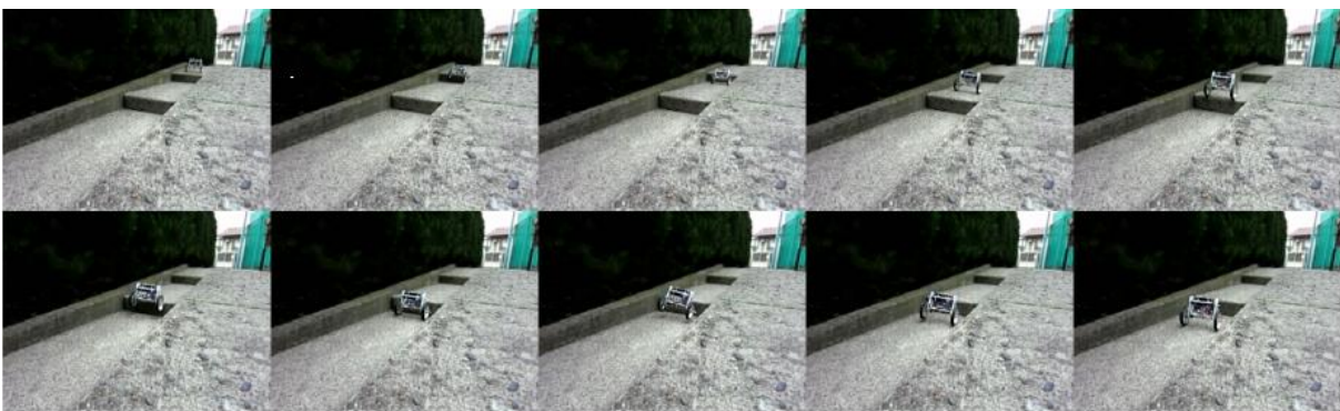
Figure 4-12: Snap shots of experiment of traversing on outdoor concrete stepped terrain
