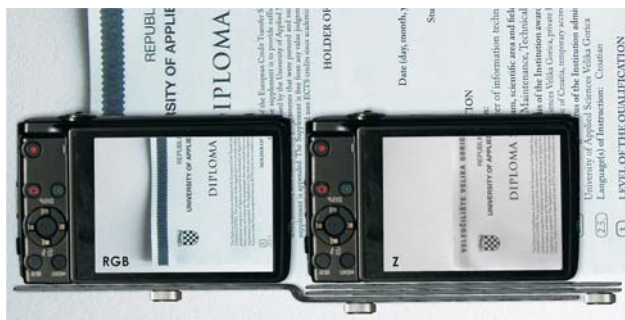
Figure 7 Highly secured document with security pattern that has a hidden text in the NIR (Z image)
