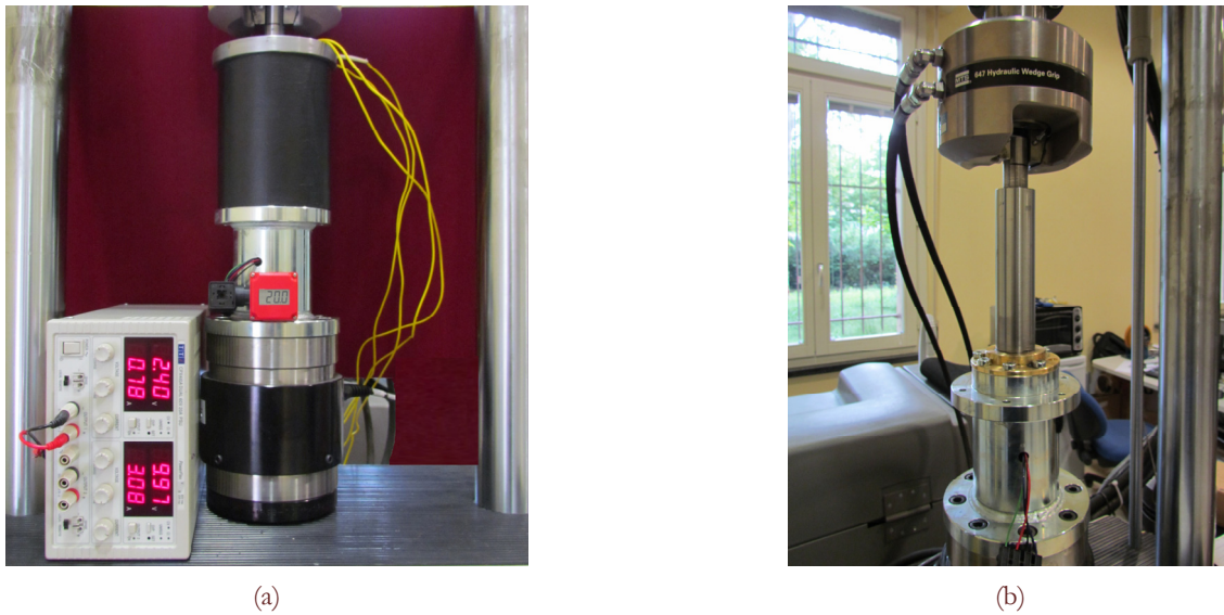
Figure 2: MR fluid insertion (a) central ferromagnetic piston fit (b) and full system mounted on the tensile machine.
