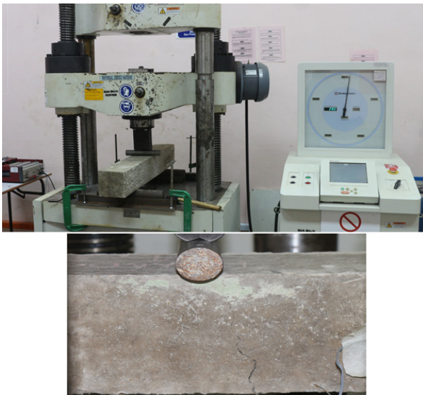
Figure 14: Failure mode for beam B2, non-fiber reinforced concrete.
