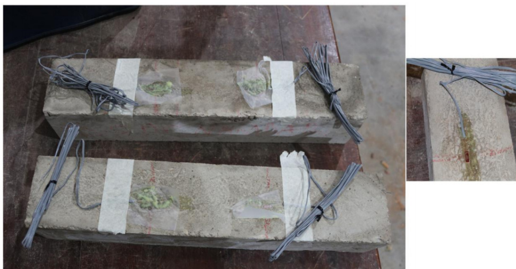
Figure 7: Strain gauges installed on concrete beam.
