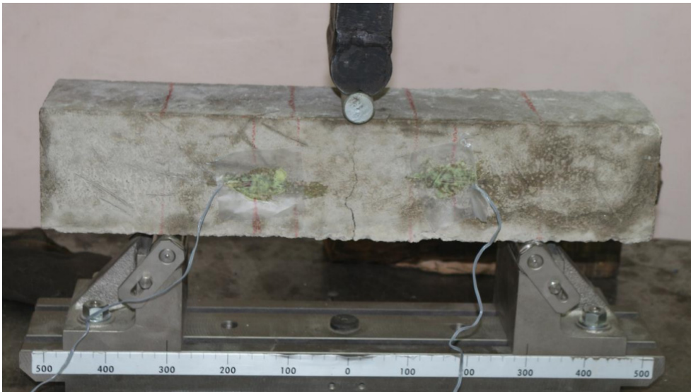
Figure 9: Failure mode for beam B1, content 1.0% steel fibers.
