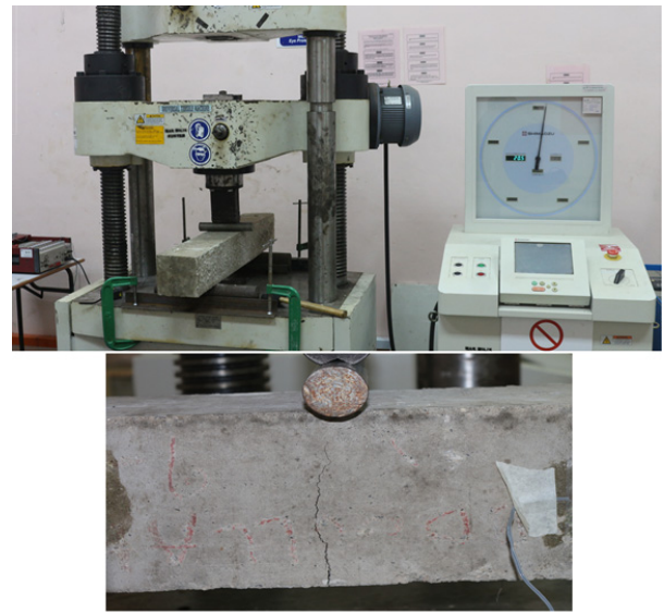
Figure 15: Failure mode for beam B2, content 1.0% steel fibers.
