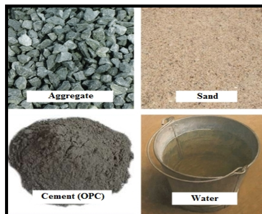
Figure 3: Basic materials of concrete.
