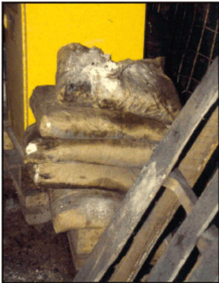
Figure 11.—Rock dust storage unprotected.
