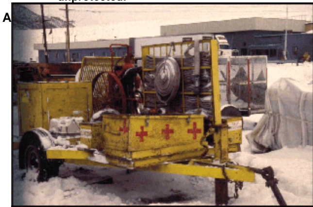
Figure 12.—Fire trailer located on the surface of an underground mine.
