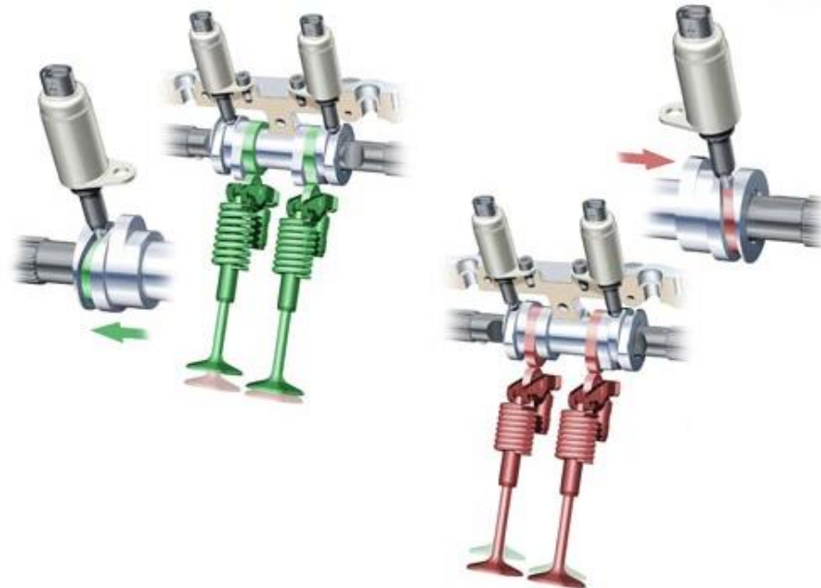
Figure 8 Audi Valvelift System [5]
