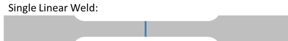
Figure 21: Position of welds on the tensile specimens
