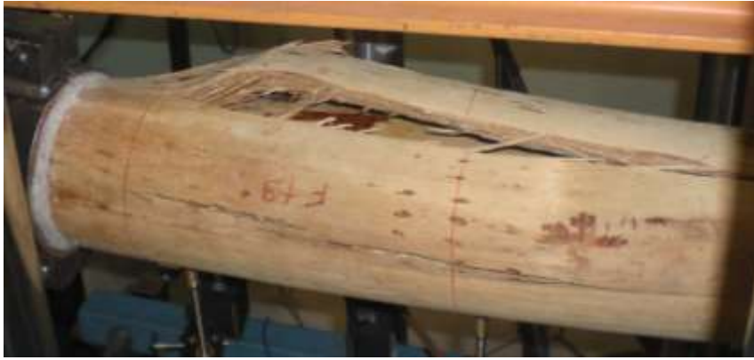
Figure 4: Failure mode for Pole 2
