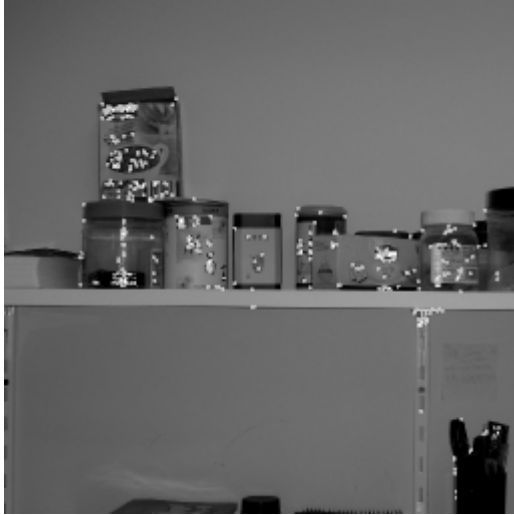
Figure 9 pattern detection with -20% luminance on office
