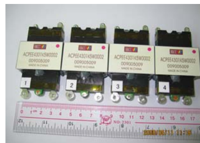
(a) Planar transformer over-view
