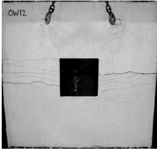
Figure 13. Wall Crack pattern of OW12
