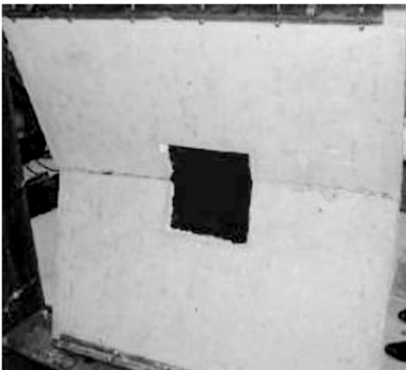
Figure 7. Crack pattern on compression face of O50W1C1.2
