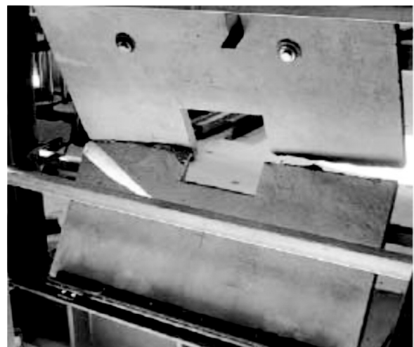
Figure 8. Crack pattern on compression face of O90W1C1.2
