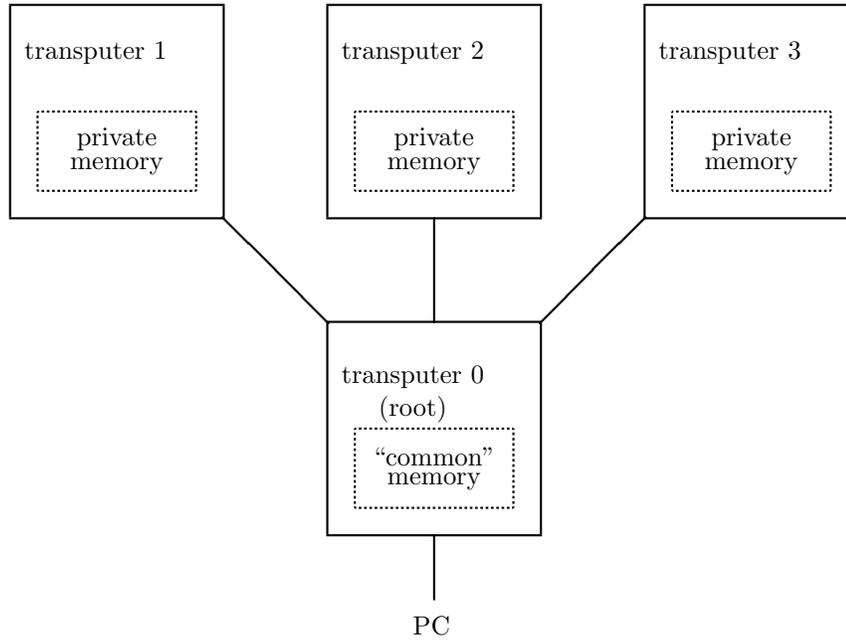
Figure 4. *Emulating a multiprocessor by a transputer network*
