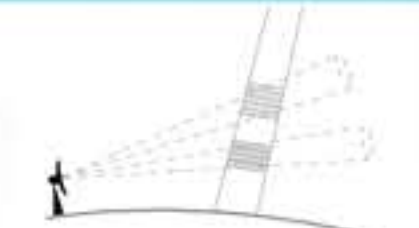
Example of DPR gate averaging of GR range interactions. Shaded areas show individual DPR gates intersecting the vertical extent of two GR ranges (shaded) at different elevation angles. The reflectivity values of the individual DPR gates are averaged over the vertical extent of the GR ranges, resulting in two matching volumes for the single DPR ray shown in this case.
