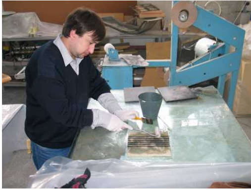
Fig. 1 - Lay up of the composite reinforced with tissue
