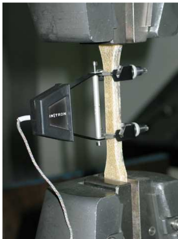
Fig. 6 - Traction test - composite tissue/epoxy
