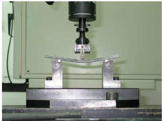
Fig. 7 - Flexion test - composite mat/epoxy
