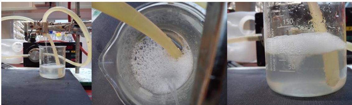
Figure 24 - Results obtained with the blank solution on the assimilating pump test method.
