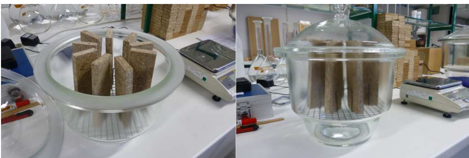
Figure 1.3.5 – Apparatus of desiccator testing, according to JIS A 1460 (on left an open desiccator with test pieces and an example of a test running at right) – (Department of Wood Engineering, IPViseu)
