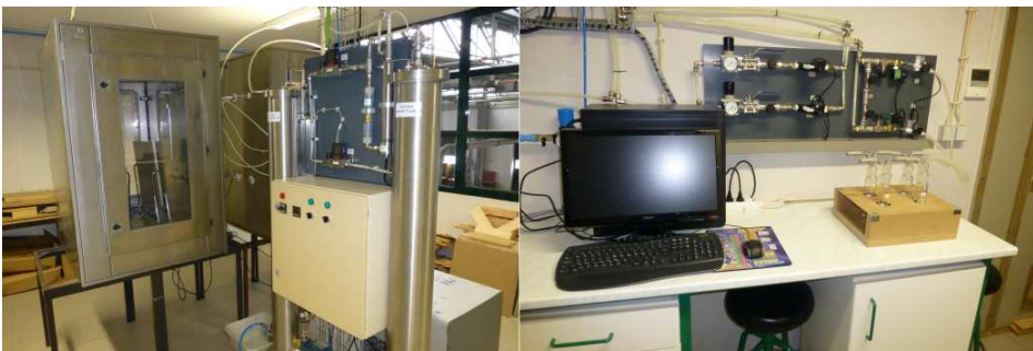
Figure 1.3.3 – Apparatus a chamber method (EN 717-1), including the chamber and air source (left) and collecting system (right) – (Department of Wood Engineering, IPViseu)
