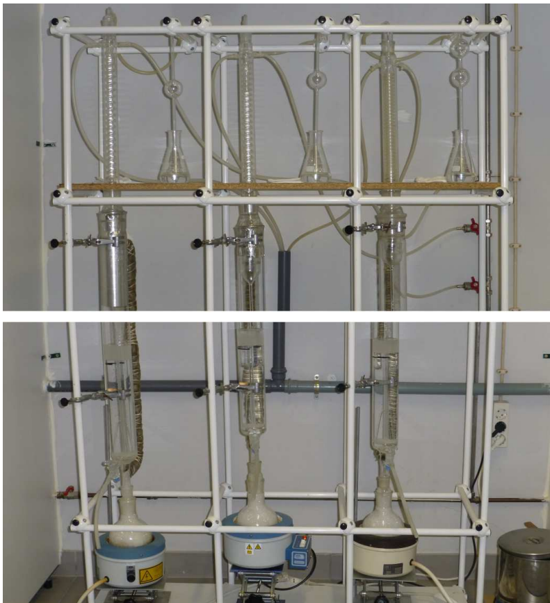
Figure 1.3.6 – Perforator equipment used in EN 120. Lower image shows test samples boiling in toluene and upper image shows the collecting system for formaldehyde dissolved in water – (Department of Wood Engineering, IPViseu)
