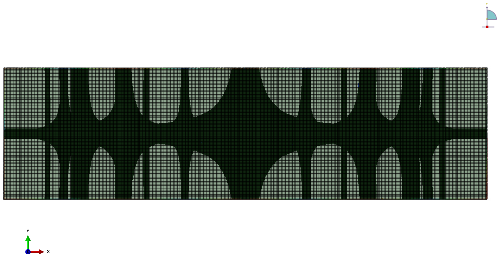
Figure 5. Nodal lines map overlapped by the mesh of the plate
