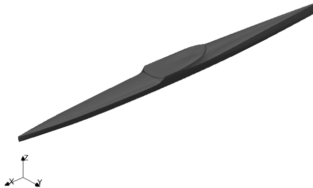
Figure 9 – Coordinate system used for all the simulations conducted, relative to the Vanquish III kayak
