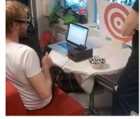
WiRe: Whiplash Rehabber uses a head-mounted laser and camera tracking to aid testing and rehabilitation of whiplash patients.
