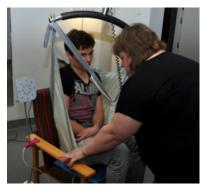
ERAIS: Ergonomic Aiding Seat enables a nurse to correctly position a patient by monitoring pressure data from the wheelchair seat, which is displayed on the LED display at left.
