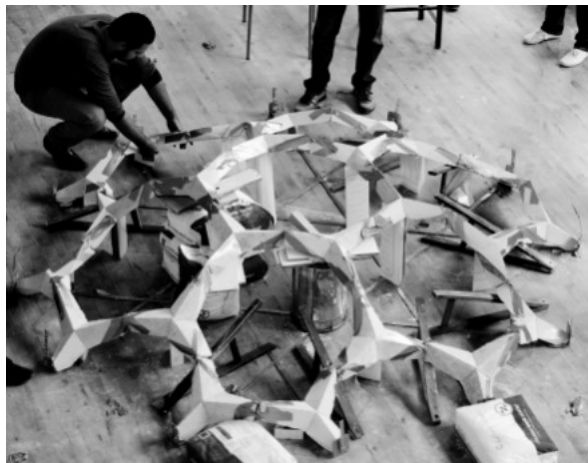
Figure 11: The 'worst-case' prototype after structural failure.
