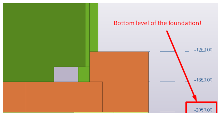
Figure 5.6: Bottom level of the foundation.
