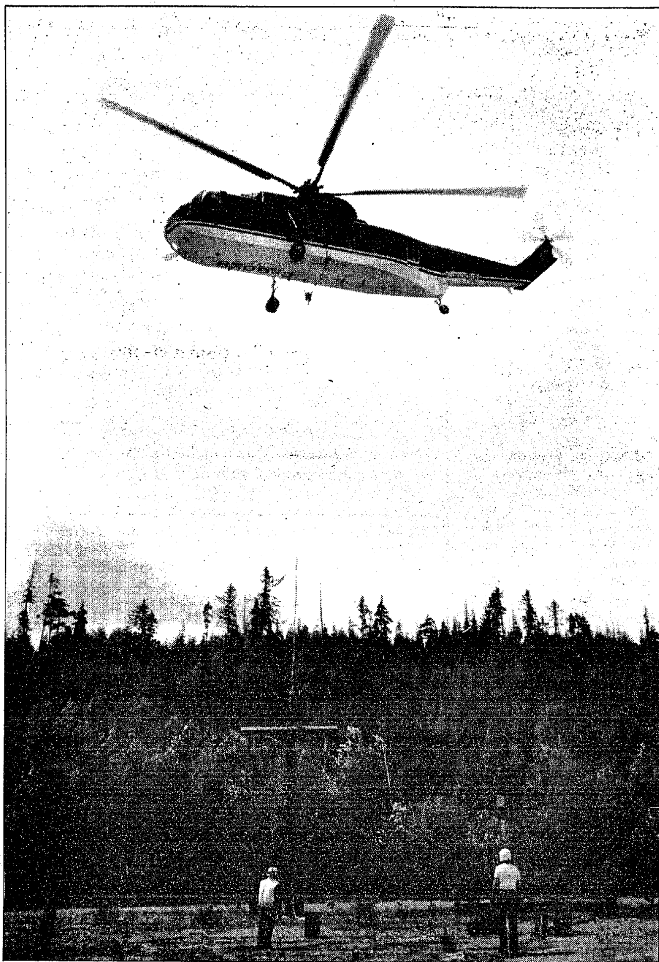
A giant Sikorsky S-61 was chartered from Canadian Helicopters by the Shames Mountain Ski Corporation to move lift towers off Kitsumkalum Mountain into the former ski hill's parking lot recently. The towers are being refitted in preparation for moving them to Shames by truck.
