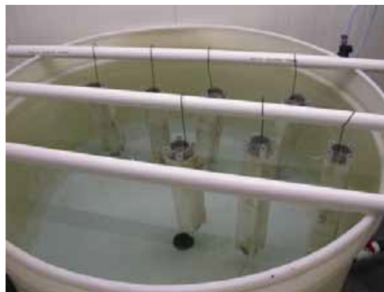
Figure 5: Wrapped collector (left) and collectors suspended in tanks (right) (Source: Edwards & Watson, 2011).
