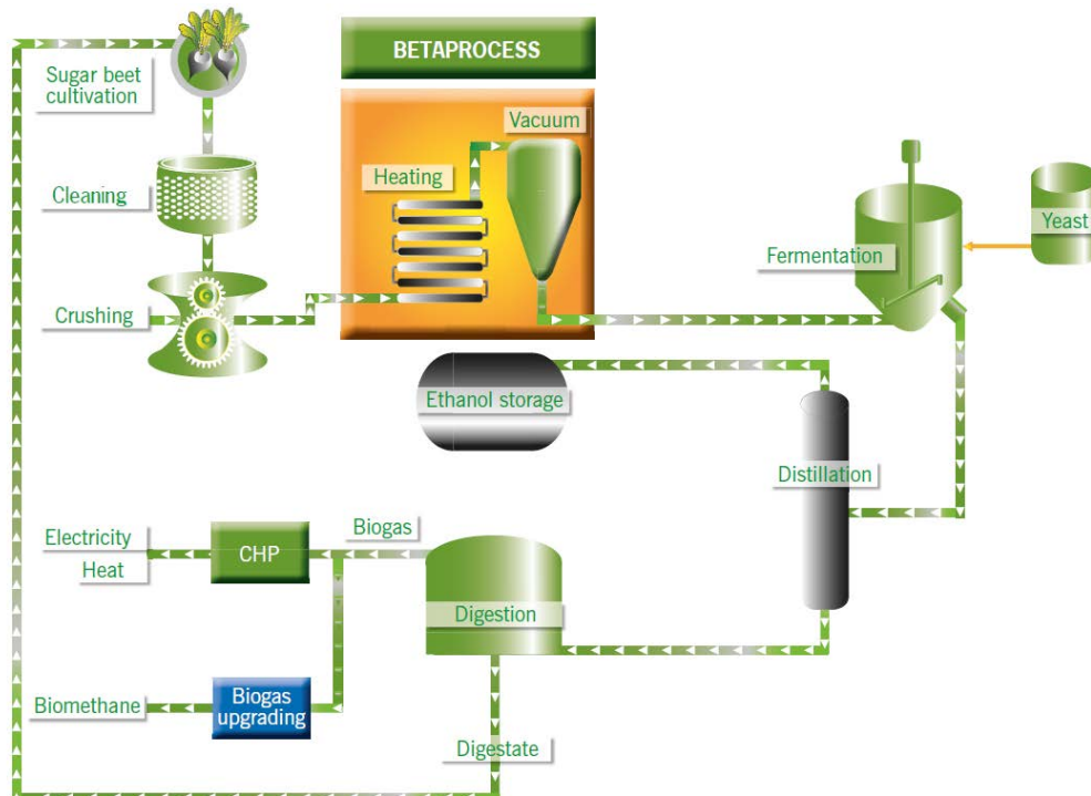
Figure 1 Schematic representation of Betaprocess integration with bioethanol pilot at ACRRES.
