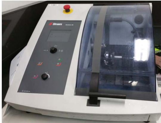
Figure 3.3: Struers Secotom cut-off machine for low speed cutting of magnesium specimens.
