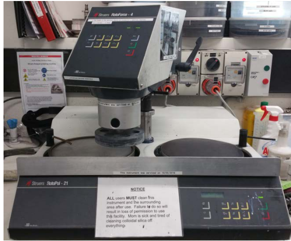
Figure 3.5: Struers RotoForce-21 grinder and polisher machine.
