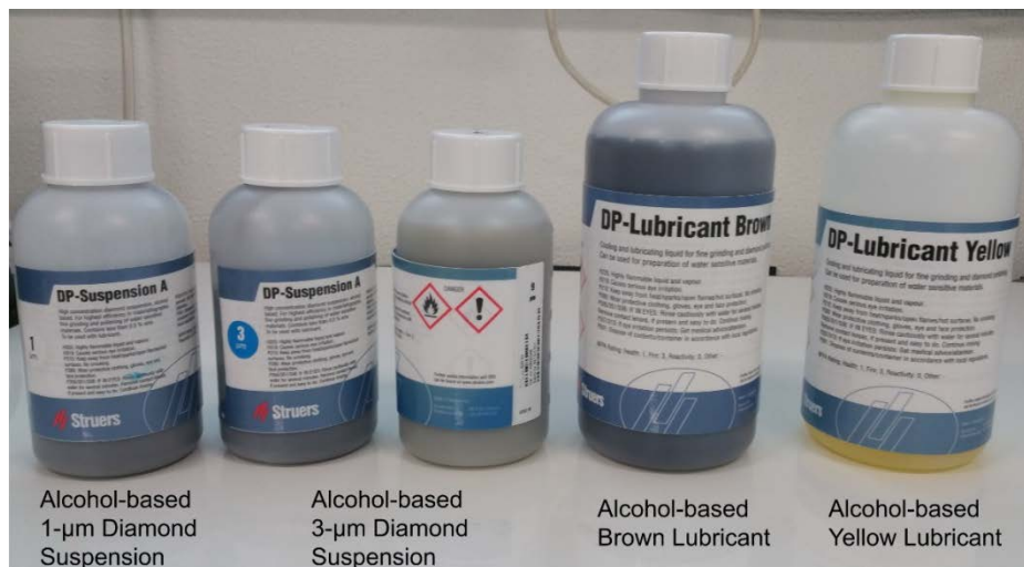
Figure 3.6: Struers lubricants and diamond suspensions used in grinding and polishing steps.
