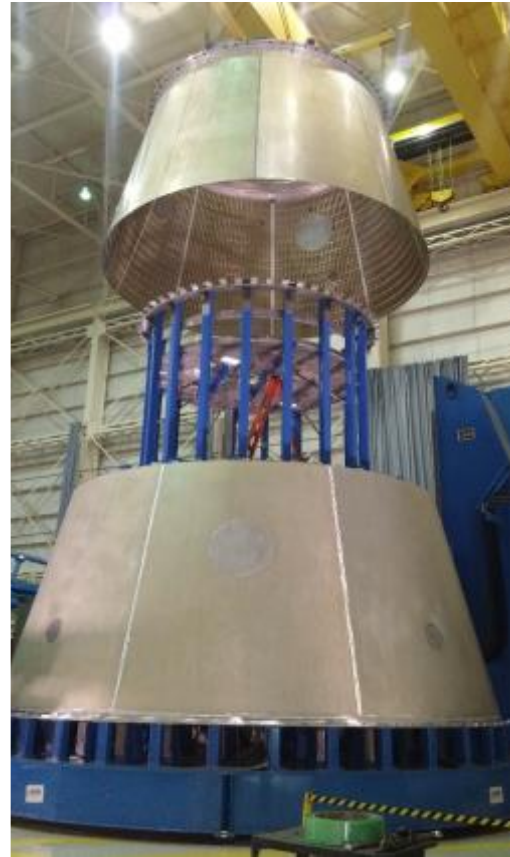
Figure 6. Joining of forward and aft cones of the LVSA.
