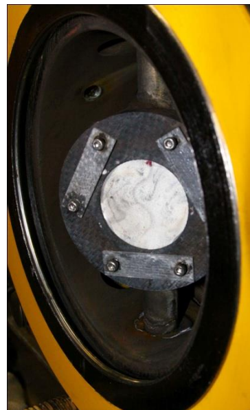
2" diameter ND3 EBC/SiC/SiC specimen after testing in the high pressure burner rig
