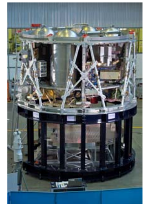
Figure 8. Structural Test Article STA-1.
