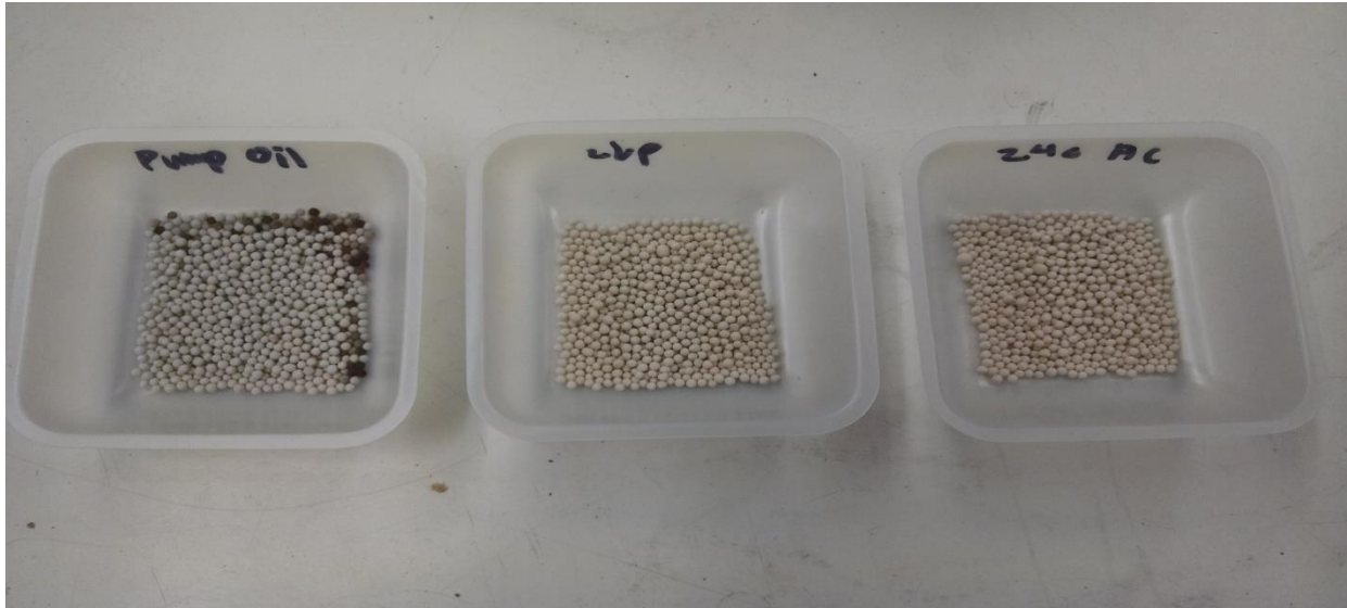
Figure 6: Chemical contamination samples after 12h 300°C bakeout. The pump oil sample shows visible greying, with some of the beads turning very dark in comparison with the LVP and 240AC samples, which did not show significant visible changes from prior to bakeout.
