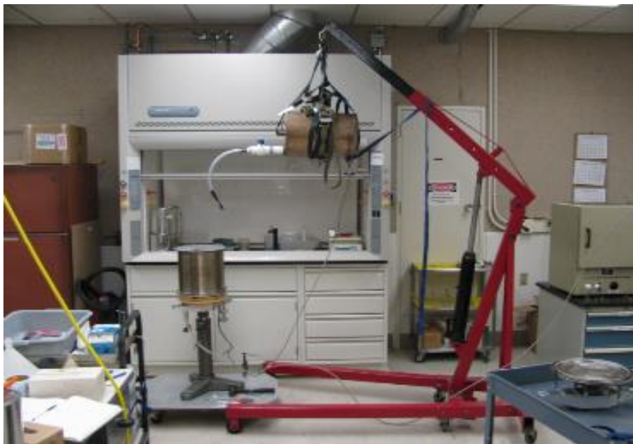
Figure 2. CRCS sorbent loading process. Bakeout canisters hoisted up by crane and manually tilted to pour sorbent. N 2 gas purge flow through bottom of CRCS and bakeout canister.
