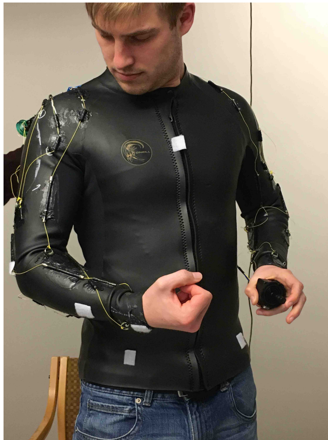
Fig. 1. CRUX: a soft, lightweight (1.3kg), robotic exosuit for upper-extremity augmentation that does not significantly inhibit flexibility of its user.
